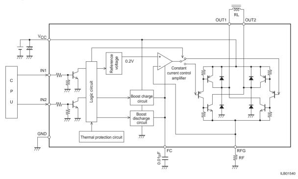
[Boost charge and discharge circuits]
